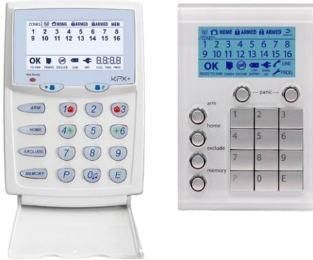
Note that some Saturn keypad models do not have CELLULAR signal and real time clock display. Operational functions are unaffected, however it's recommended that at least one KPX+ keypad be installed to provide cellular signal indication.
