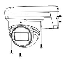
Adjust the camera's position and angle by loosening the lock screw at the base of the camera. When the camera's desired position is achieved, secure the lock screw back in place to complete the installation. For vandal dome cameras, complete the installation by placing the dome cover on the camera. Secure the dome cover to the camera base using the screws included with the camera. See the camera's QSG for more information.
